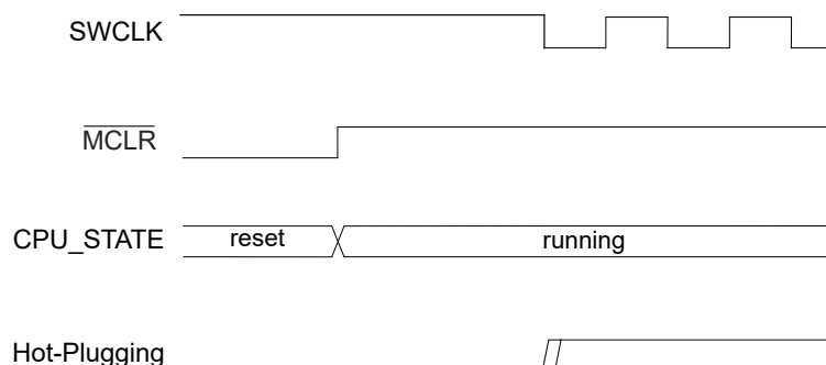
Figure 16-3. Hot-Plugging Detection Timing Diagram
